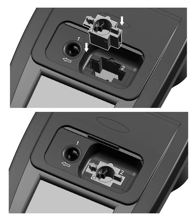
Figure 5 Installation of a cuvette/sample cell adapter
